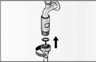
4. Carefully turn on the tap and check that the connection points are not leaking.
