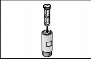
2. Place seal in the filter housing and connect to the tap (3/4" threaded connection).
