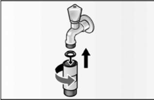
3. Using an open-end wrench, connect water supply hose with seal to the filter housing (if not already fitted ex works).
