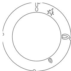
On the front panel, above each knob, the burner it corresponds to is indicated by the index
